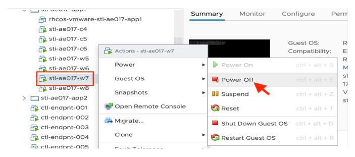
Figure 5 Powering-off a worker node (VM) to simulate Apache Cassandra Cluster node failure
