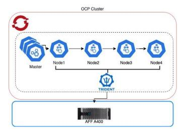
Figure 1 RedHat OpenShift Container Platform cluster config view
