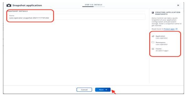
Figure 11 On-demand application snapshot in NetApp Astra Control
