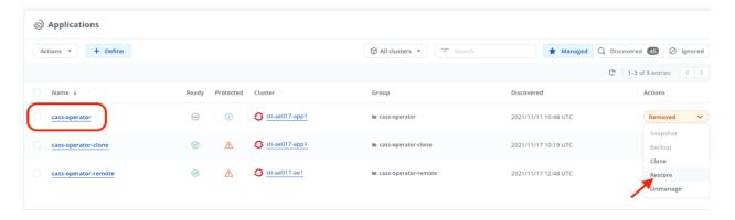
Figure 26 Restoring Apache Cassandra from a backup using NetApp Astra Control
