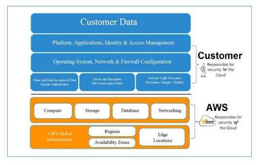
The above image shows that anything below the hypervisor level, including hypervisor security, servers, racks, power supply, and the Internet, is completely the responsibility of the cloud provider (that is, AWS). Anything above the hypervisor (that is, the operating system, network, firewall configurations, applications, and encryption) **is completely your responsibility**.
