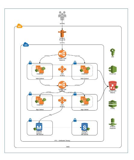
In the above HIPAA-compliant architecture, Amazon VPC with dedicated tenancy is used. All traffic is encrypted in transit with SSL termination, and back-end authentication is enabled at the ELB layer. The communication between the web layer and app layer is also encrypted with an internal ELB layer used between them. All the instances in the web layer and app layer are using KMS-encrypted EBS volumes. The database is again encrypted using AWS KMS service.
