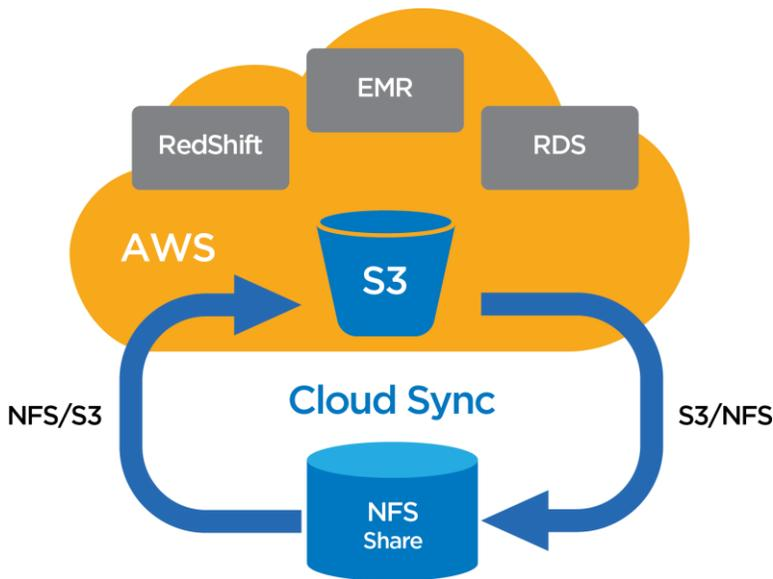
Cloud Sync rapidly moves datasets to and from AWS, converts file-based NFS datasets to the S3 object format, and can launch various cloud services, including EMR or RDS.
