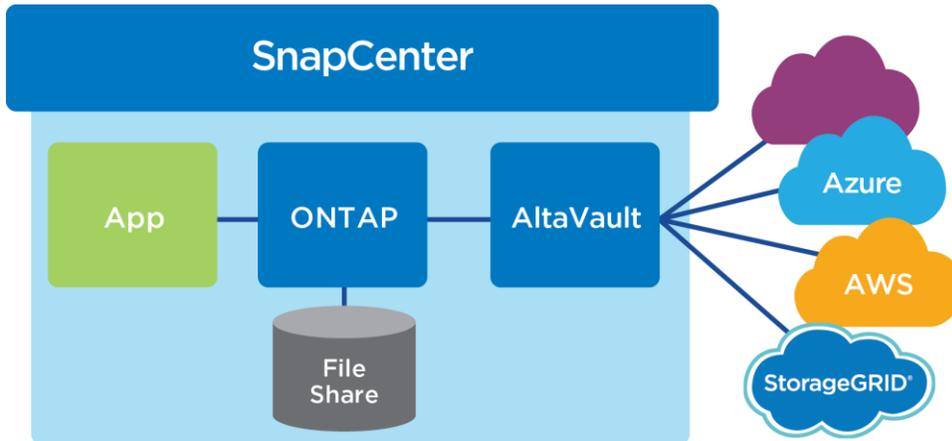
The ONTAP and AltaVault endpoints are integrated using the SnapMirror data protocol, allowing for fast and efficient data transfer between them. This integration allows endless incremental backups after creation of the first complete baseline.
